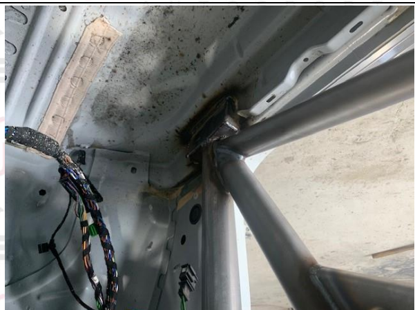
PHOTO 6 FRONT ROLLBAR TO FLOOR ATTACHMENT
