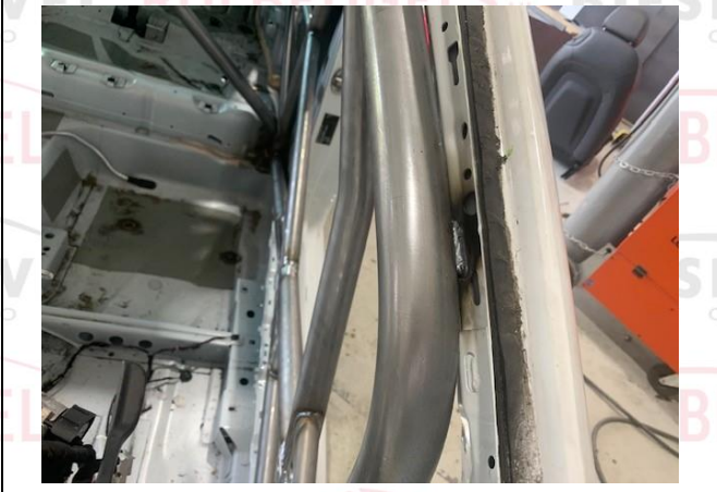
PHOTO 7 FRONT ROLLBAR TO "A" PILLAR ATTACHMENT
