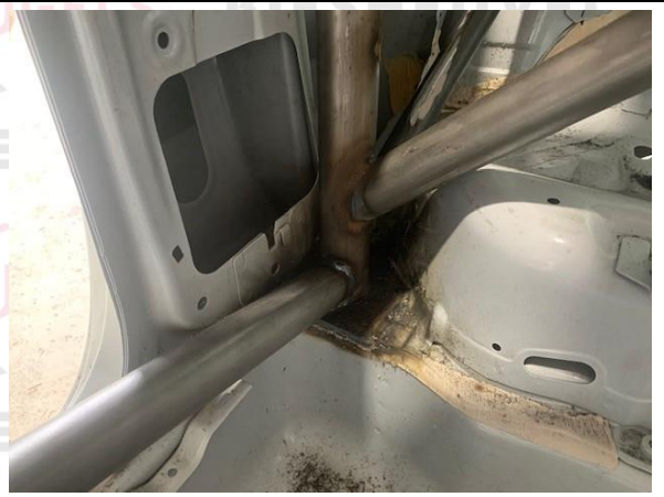
PHOTO 4 MAIN ROLLBAR TO FLOOR ATTACHMENT
