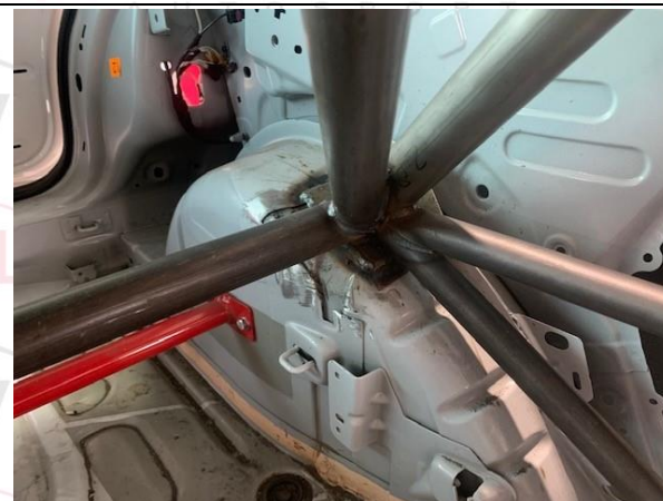
PHOTO 5 REAR BACKSTAY TO BODYSHELL ATTACHMENT
