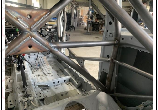
PHOTO 13 SHOULDER HARNESS ATTACHMENT - CO DRIVER
