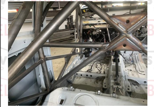
PHOTO 12 SHOULDER HARNESS ATTACHMENT - DRIVER
